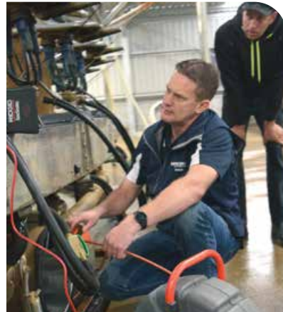
Daviesway DASCOS Shaun Kingston (Tasmania) can check the entire milk line within minutes with an in-line camera. Daviesway DASCOS's service is free for its chemical customers.
